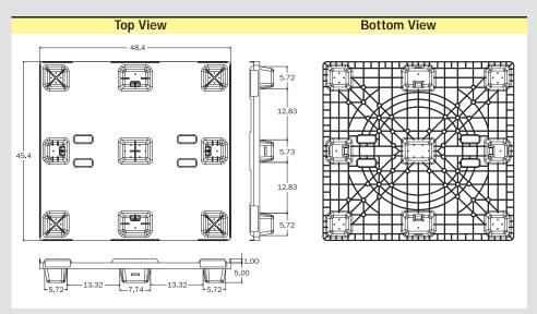
Though Krypto-Lite is shown, above dimensions apply to both the Krypto-Lite and AF Pallet.
