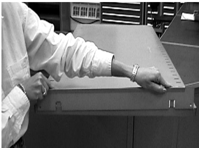
Position tabs on Shelf Guides over slots on ends of each Shelf and drop in.
